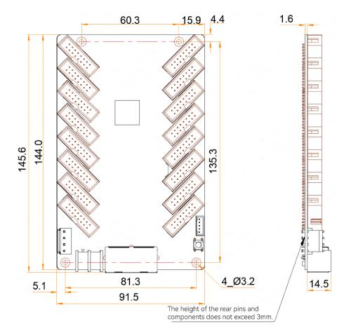
Tolerance: ±0.3 Unit: mm
